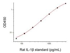
Figure 1. Standard Curve of Rat IL-1 $\beta$  in 96-well plate assay, data provided for demonstration purposes only. A new standard Curve must be generated for each assay.
